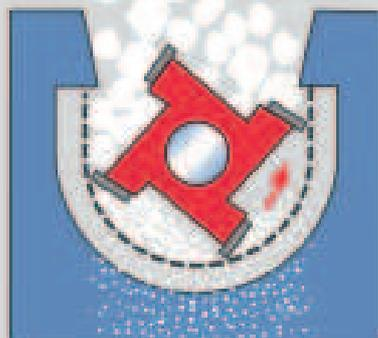
use a hole size of at least 10 mm in order to avoid clogging. For applications with a tendency to agglomerate or be greasy, Gericke uses a mesh sieve to prevent blockage. The slight vibration in operation further supports this. The distance between the paddles and the screen is decisive for efficient operation, both in the case of the basket and of the sieve. It depends on the properties of the product to be processed.
