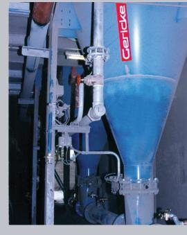
This Gericke dense phase conveyor, reduces the air requirements by 45-50% when compared to other systems. Utilising existing compressors, it was possible to increase the conveying capacity threefold. The low conveying speed reduces wear to an absolute minimum and the unique Gericke pipebends allow virtually abrasion-free diversion of the product flow. The Gericke twin-transmitter system ensures maximum conveying efficiency with high output, low air consumption and minimum maintenance.
