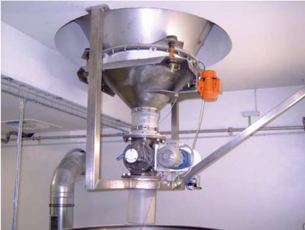
Gericke vibrating bin activator and rotary valve for feeding product into the sieve
