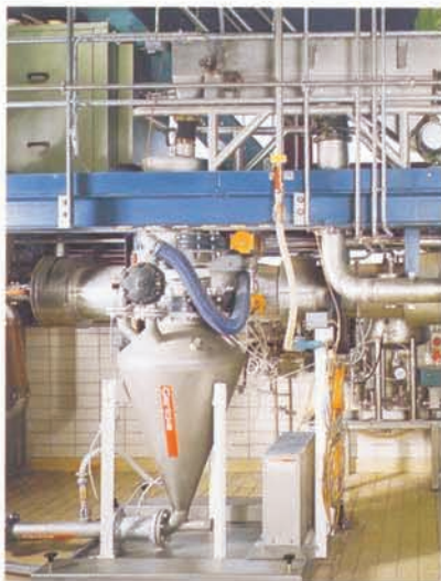
This chemical production dense phase conveyor incorporates weighing and recording of the throughput.
