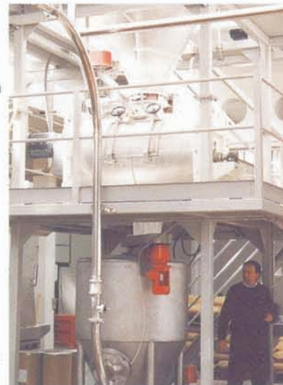
Ploughshare mixer plant for the pre-mix of confectionery ingredients
