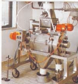
This chemical production dense phase conveyor incorporates weighing and recording of the throughput.
