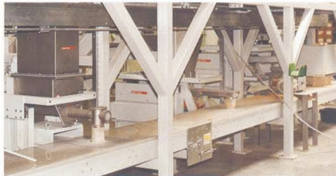
Feeding and mixing system for the preparation of muesli. Ingredients are transferred from the weigh feeder by an enclosed belt conveyor to the continuous mixer.
