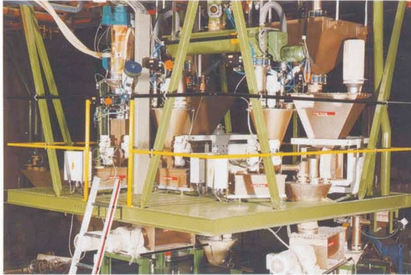
Continuous feeding and mixing system into an extruder for the production of plastic tubes. System includes weighfeeders and continuous mixers for 8 ingredients.
