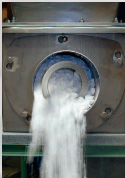
The paddles press the filter cake through the screening plate, the advantage being that the filter cake is cut up without producing many fine particles. This is a very efficient way to fill drums, for example.
