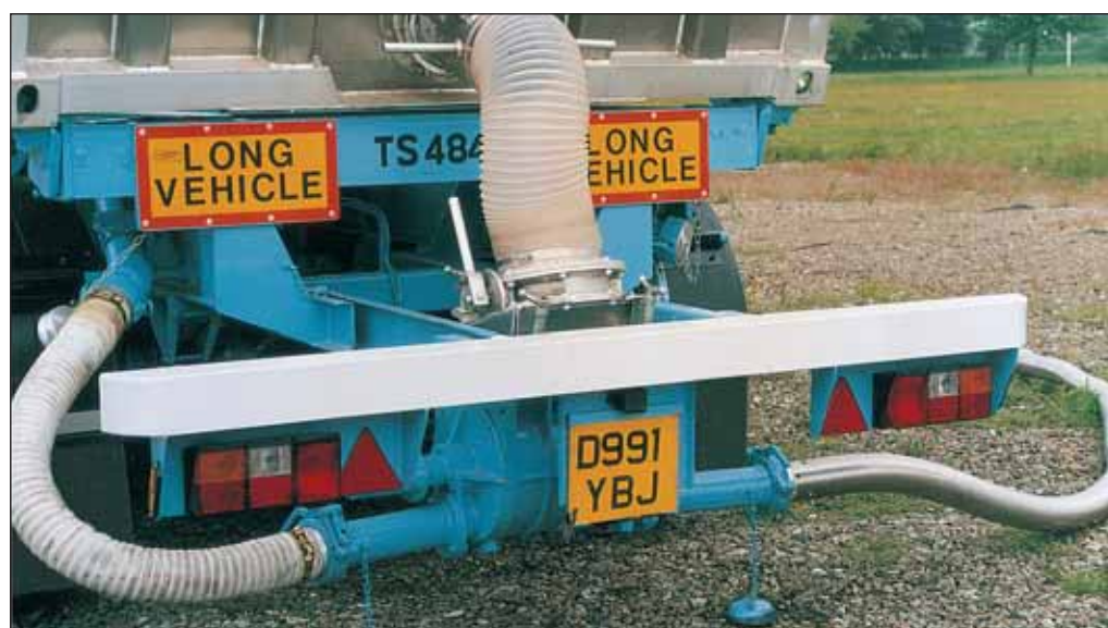
Mobile bulk container emptying unit with Rotaval® rotary valve.
