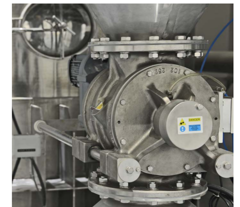
Rotary valve discharge
