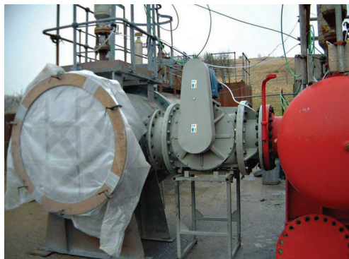
FIGURE 3. 600mm bore valve undergoing ATEX testing (For explosion/flame containment validation by Notified Body)
