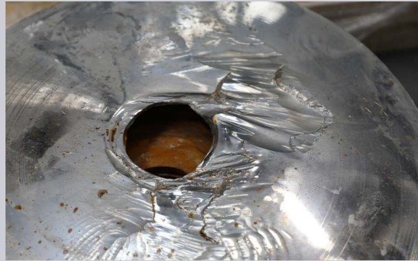
Abrasion caused by pigments in a rotary valve. Heavy-duty and modular rotary valves simplify maintenance in such plants.
