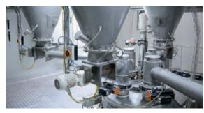
Direct dosing into the reactor
