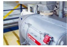
Mixing in a mechanical fluid bed
